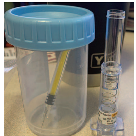
Figure 1. When attempting to engage the safety mechanism on an enoxaparin syringe (Fresenius Kabi), the two pieces completely separated from each other.
