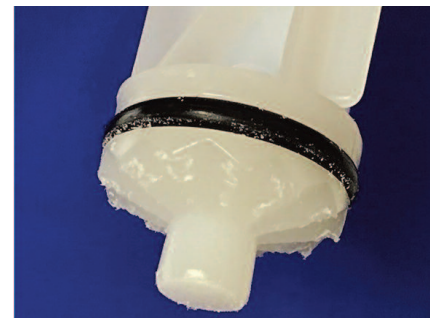
Figure 1. Plunger's teeth broke when used with a hard-to-crush tablet.
