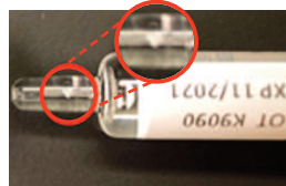
Figure 3. Silicone core appears in nozzle of Dr. Reddy's naloxone prefilled syringe.
